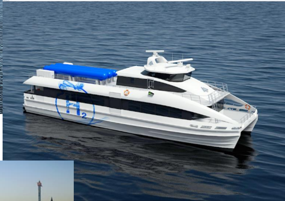
Water-Go-Round, first fuel cell / H2 gas vessel in the US (Golden Gate Zero Emission Marine, 2019)
